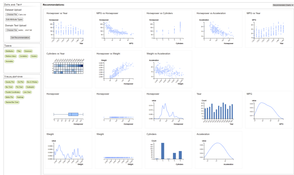
Figure 4. The TaskFinder interface that takes in a dataset along with related textual documents via inputs on the top left and produces a set of recommended visualizations that can be used to explore the most important features of the data. Users can control the recommendations by selecting the tasks they are interested in and the visualizations they are familiar with via the task and visualizations panels on the left.
